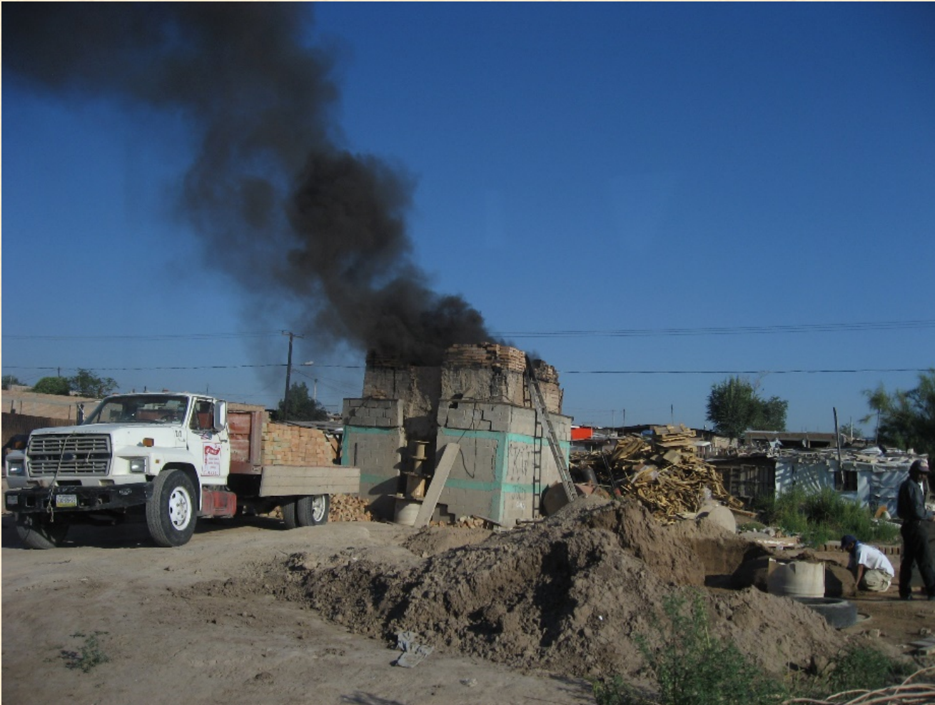
Traditional brick kiln burning scrap materials—scrap wood, sawdust, tires, battery cases, plastics, particle board, used motor oil—near homes and businesses in Ciudad Juárez
