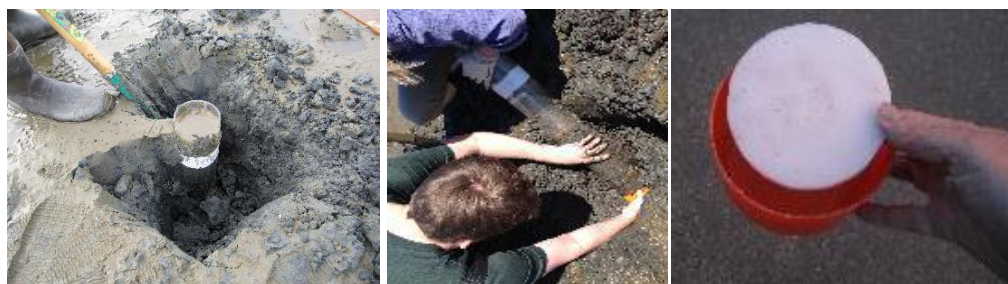
Figure 19. Excavating sediments around core tube to facilitate removal. A plastic disc and plumbing end cap are positioned over the lower end of coring tube.
