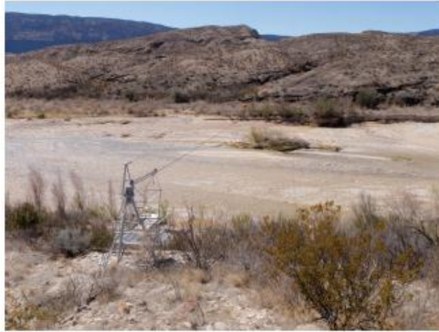
Figure 3.2-4. Photo of the Terlingua Creek gage and cableway. Photo is taken from left bank and flow is from right to left.
