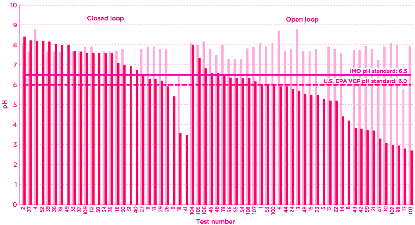
Figure 3. pH in scrubber discharge water. Gray bars show pH values before entering the scrubber system; orange and red bars show pH values after scrubbing process for closed- and open-loop scrubbers, respectively. Blue line indicates a pH of 6.5, consistent with IMO guidelines, and the purple dashed line is equal to a pH of 6.0, consistent with EPA 2013 VGP.
