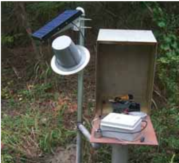
Figure 4.3 Monitoring well with satellite telemetry equipment.
