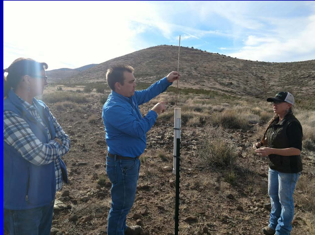
PVC depth gauge at range monitoring site near Clifton, AZ
