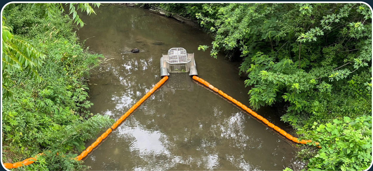
Osprey Initiative installed traps, including the Litter Gitter pictured above, at 3 sites in Davenport: Goose Creek at the Gaines/Scott Pedestrian Bridge, Silver Creek at 49th Street, and Duck Creek at Marquette Street. Source: Osprey Initiative
