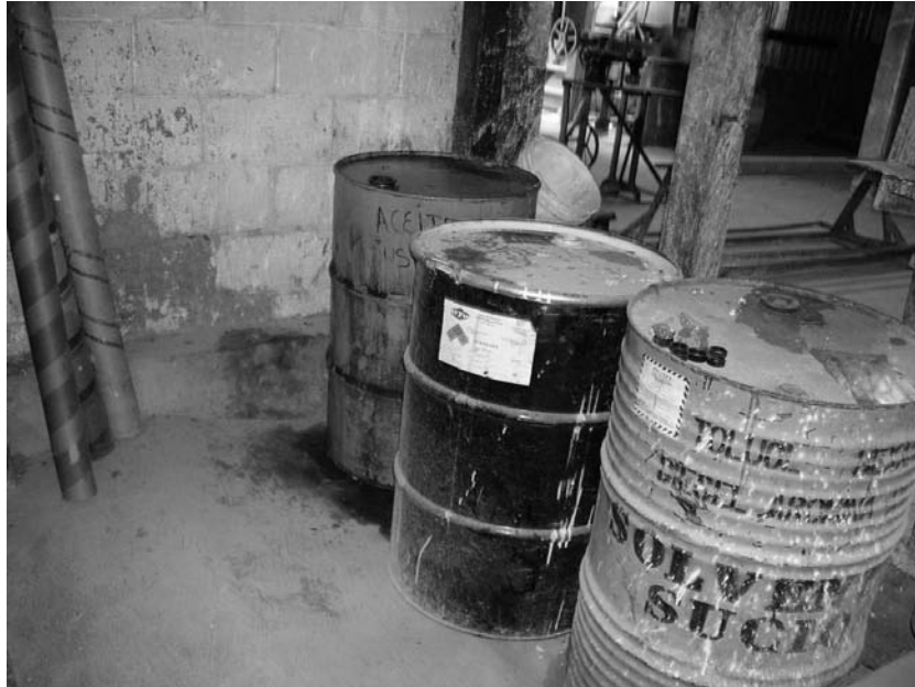
Photo No. 9: Area for storing hazardous wastes. Drums with solvents and used oils were observed there.
