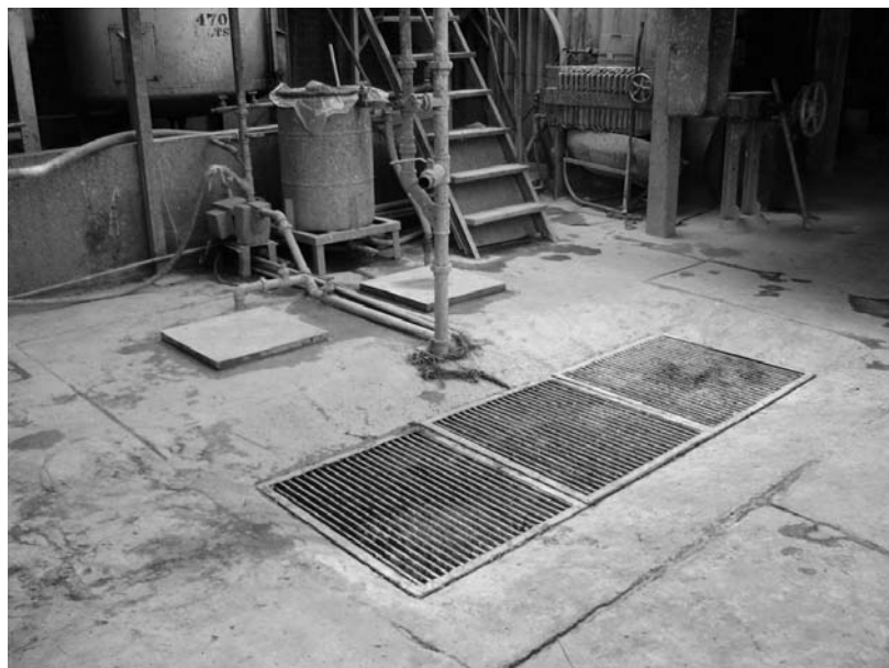
Photo No. 6: View of the outdoor area where the activator was prepared. The process was conducted in the open air. Also visible is a screen for catching any product spilled.
