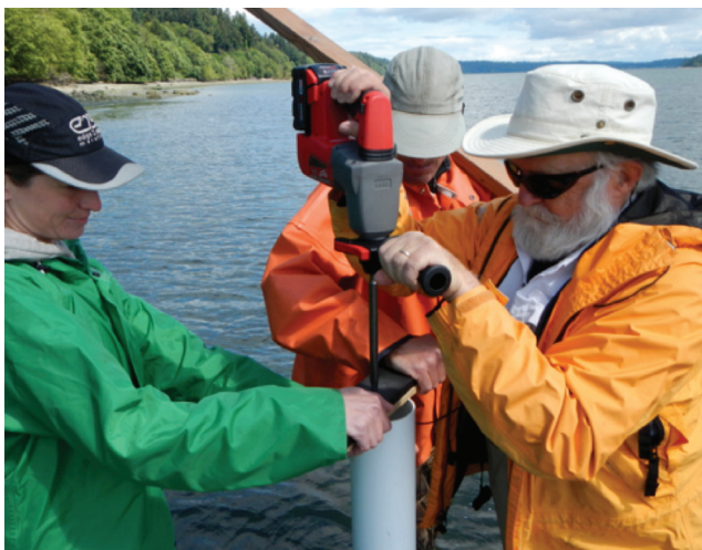
Figure 4. Sediment coring with a hammer drill
