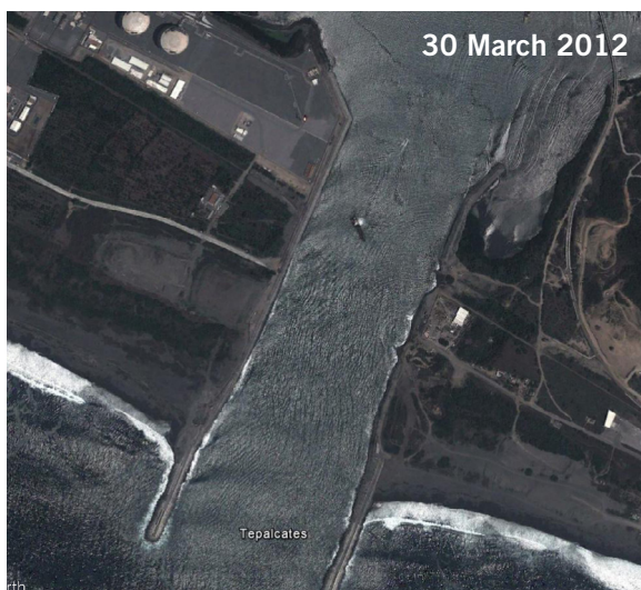
The image from 13 June 2011 shows progress on the dredging of the canal, while the image from 30 March 2012 shows the canal after dredging and the Manzanillo LNG project.
