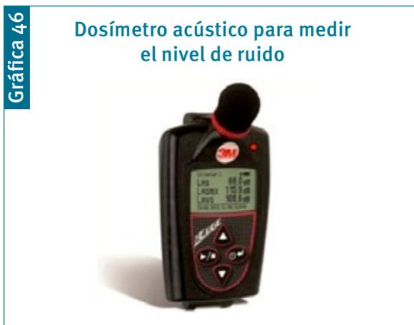
Fuente: 3M (2015), "3M™ Edge™ Dosimeters", en: <[http://solutions.3m.com/wps/portal/3M/en\\_EU/PPE\\_SafetySolutions\\_EU/Safety/Product\\_Catalogue/~3M-Edge-Dosimeters?N=5158380+3294411297+3294857473&rt=rud](http://solutions.3m.com/wps/portal/3M/en_EU/PPE_SafetySolutions_EU/Safety/Product_Catalogue/~3M-Edge-Dosimeters?N=5158380+3294411297+3294857473&rt=rud)>.
