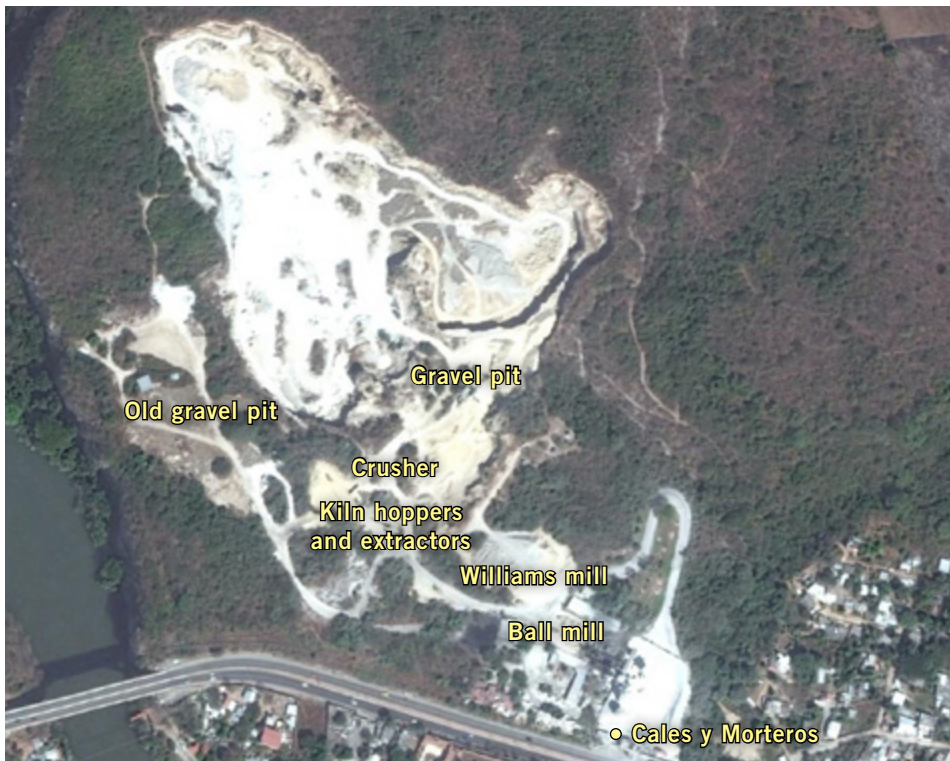
Figure 7. Distribution of equipment on the premises of Cales y Morteros 101
