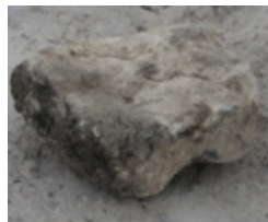
Burnt lime from the kilns (quicklime)
