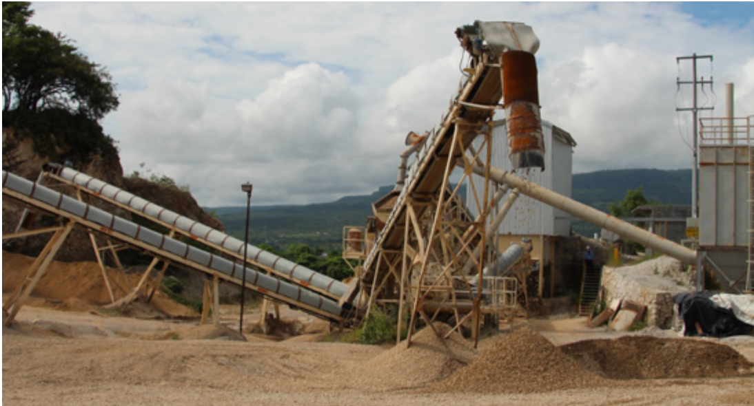
Photo 3. Screening and separating process 100
